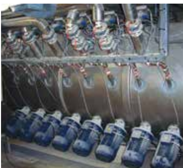
Choppers, liquid injectors, temperature jacket
